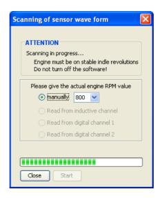
• *Preview* - feature which enable us to check the shape of scanned sensor signal wave.
